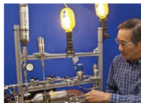
A system incorporating a fuel cell and light-weight hydrogen storage material. Credit: Savannah River National Laboratory.
