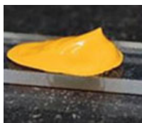
This paste of cadmium sulfide-coated titanium dioxide nanoparticles could turn large surfaces into solar cells. Credit: ACS Nano .
