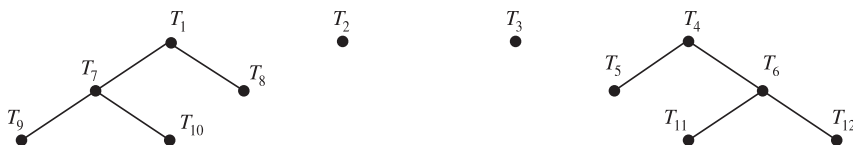
Figure 3.5. Forest \mathcal{F}_2 corresponding to the grid sequence \{\mathcal{T}_k\}_{k=0}^2 of Figure 3.4. The roots of \mathcal{F}_2 form the initial mesh \mathcal{T}_0 and the leaves of \mathcal{F}_2 constitute the conforming bisection mesh \mathcal{T}_2 . Moreover, each level of \mathcal{F}_2 corresponds to all elements with generation equal to the level.
