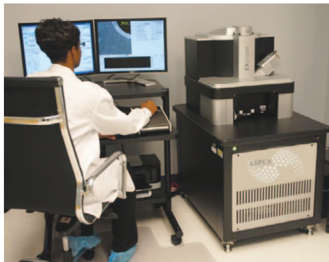
Figure 2: Laboratory technician using scanning electron microscope with energy dispersive spectrometer available for purchase by the customer. Contracted experts at the manufacturer's laboratory can analyze data quickly and efficiently using advanced knowledge of cutting-edge technology.
