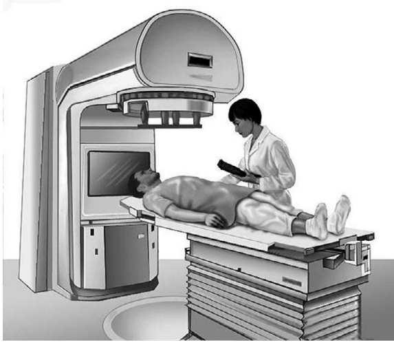
Figure 1.1 A linear accelerator machine for external beam radiotherapy. Radiation beams emerge from the top of the machine and pass through the patient's body. Source: National Cancer Institute, www.cancer.gov/about-cancer/treatment/types/radiation-therapy/external-beam and https://visualsonline.cancer.gov/details.cfm?imageid=9413 . Reused per policy available at www.cancer.gov/policies/copyright-reuse .
