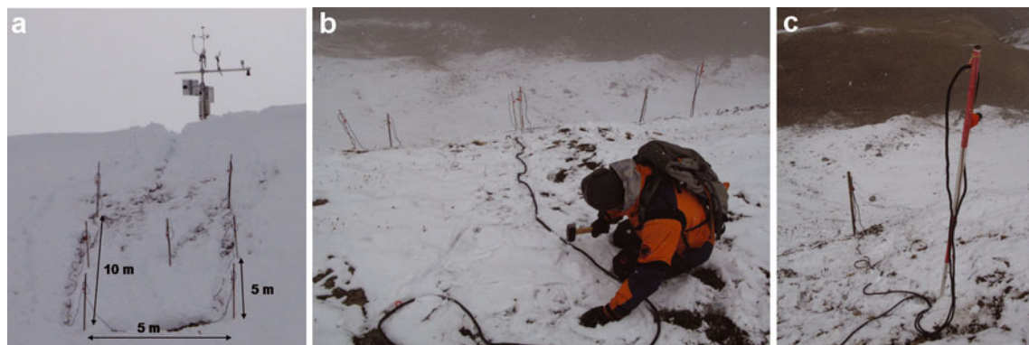
Fig. 4. The first stage of the deployment of the sensor array. (a) The deployment configuration for the winter of 2009/10. (b) Before the first major snowfall the cables of the data acquisition were fixed to the ground. (c) Wooden posts were installed on the ground surface to find the location of the geophones once the cables were covered by snow.
