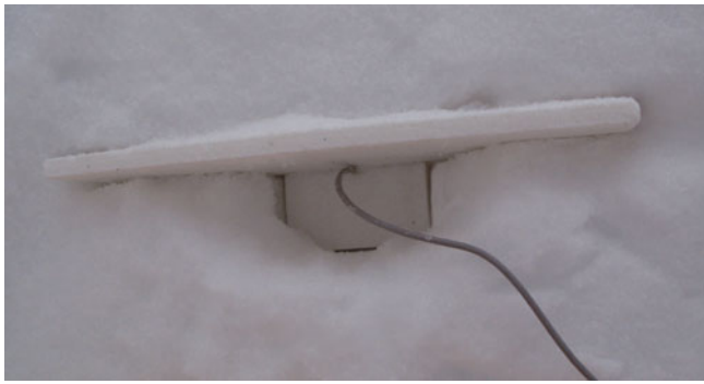
Fig. 3. Geophones inserted in the snow cover were installed in a foam housing. The foam housing improves the coupling between the sensor and the snow cover.
