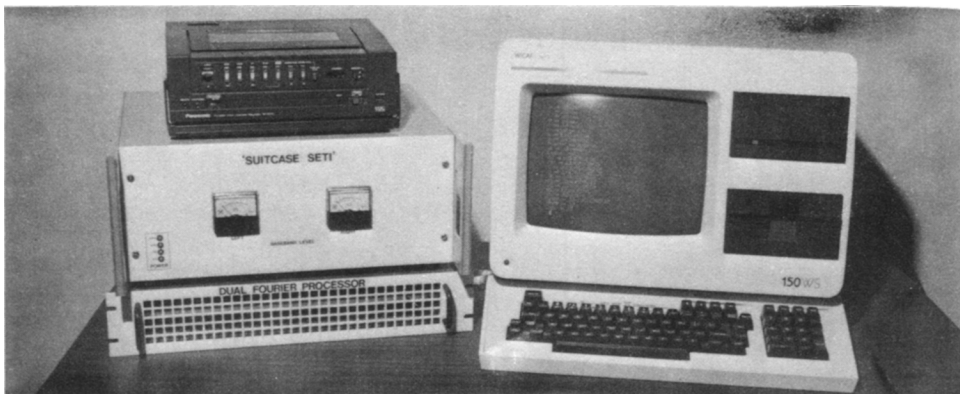
Figure 4. "Suitcase SETI": A portable multichannel receiver with real-time signal recognition and archiving.
