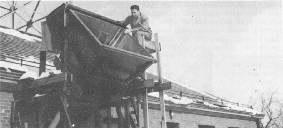
Figure 7. Harold ("Doc") Ewen and the historic Harvard antenna that first detected galactic 21cm radiation.
