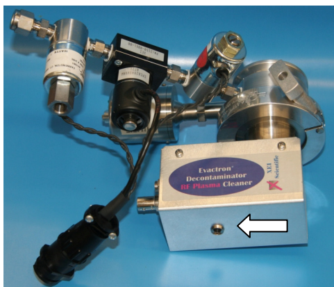
Figure 1: Old impedance matching network, or match (silver box with label) attached to valve and pressure gauge assembly. The arrow points to the trimmer cap needed for tuning of match by user.
