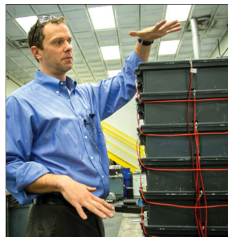
The battery stack serves as the fundamental building block of Jay Whitacre's aqueous hybrid ion systems.
