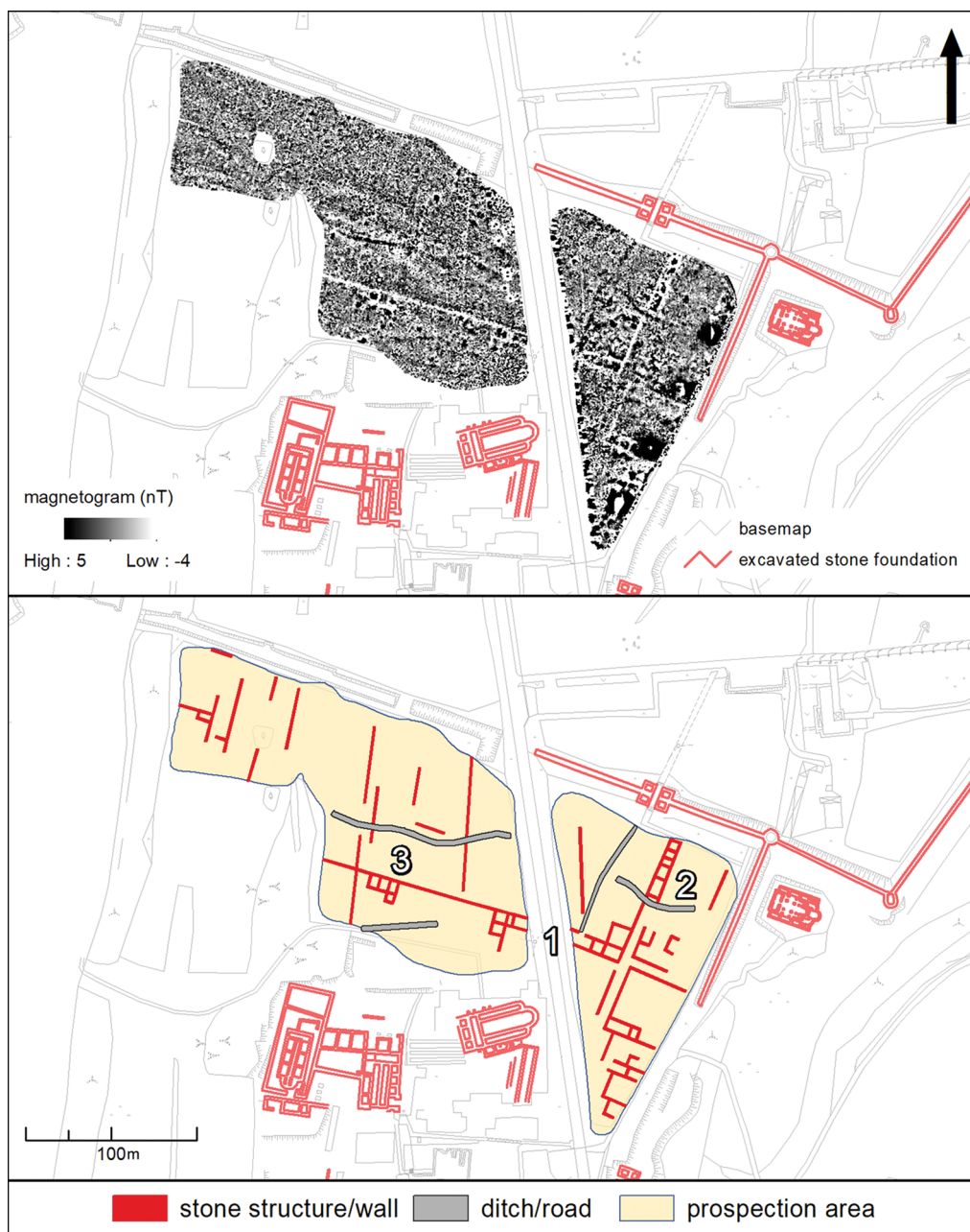
Figure 3. Veliki Preslav: Inner City (Area 1), showing the results of the geomagnetic survey (top) and its archaeological interpretation (bottom). Numbered structures mentioned in the text are labelled accordingly (figure by the authors).
