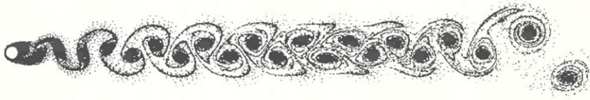
Figure 3. DVM simulation of the wake of a circular cylinder Re = 200 , S_t = 0.196 , C_D = 1.22 , G_{Arkellz} .
