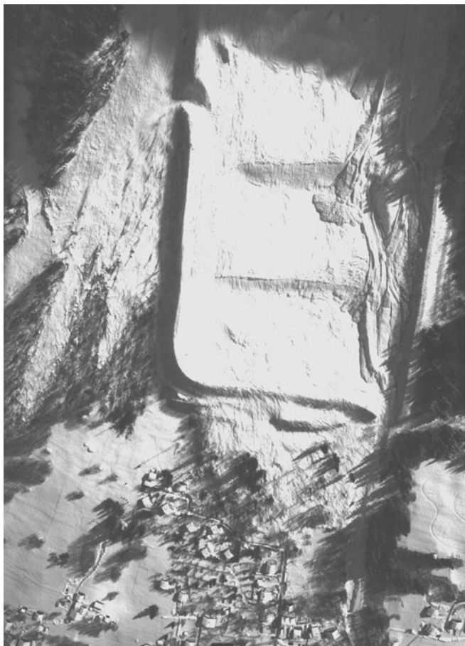
Fig. 1. Photograph of the February 1999 avalanche deposit at Taconnaz, showing the lateral and frontal overflows.
