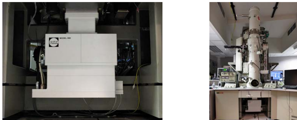
FIG. 1. US 10000 XP / model 990 10k x 10k camera installed on a JEOL 3200 FSC TEM at the National Center for Macromolecular Imaging (NCMI), Baylor College of Medicine, Houston, Texas. The camera fits within the unmodified kneewell shield (removed in these photos).
