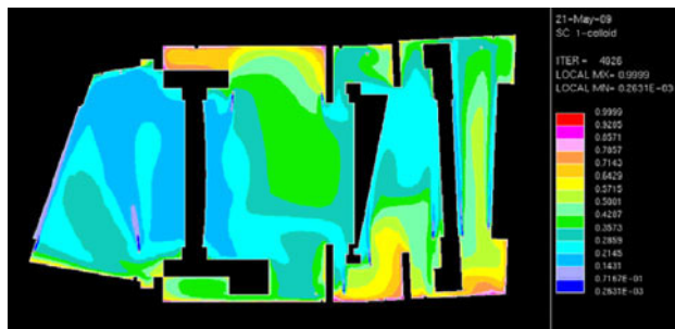
Figure 4. Density distribution of the contaminants in cross-section 2 as the flux ranges within 1–5 l s -1 after 30 s.
