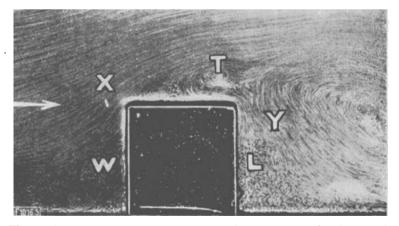
Fig. 3. Flow past model house with flat roof. Lettering on the photograph has been added by the author.
