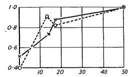
Text-fig. 4. Dependence of influx rate on area of opening at base of flue. (Averages for all observed wind velocities.)
