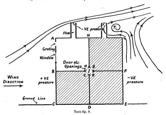
is negative, and the flue effect in each room and the negative pressure over BC will produce a negative pressure at I. The pressure on each side of a will be negative and the pressure difference and therefore the flow through a will be small.
