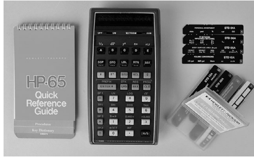
Figure 14.5 An HP-65 with its quick reference guide and magnetic program cards. Image © Whipple Museum (Wh.4529.227A).
