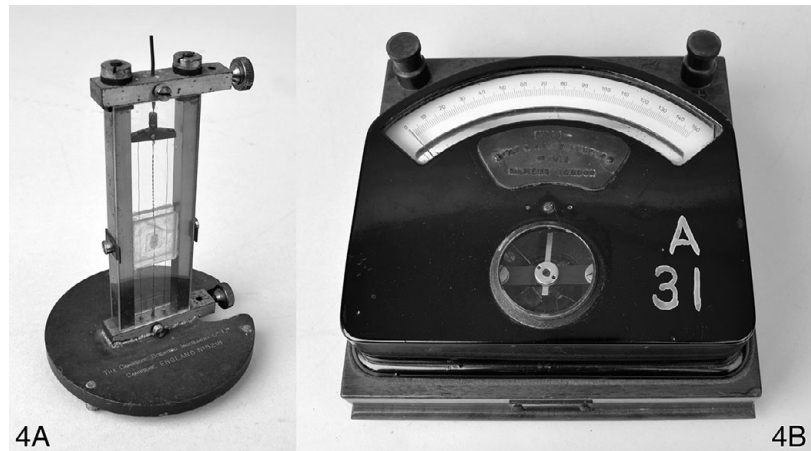
Figure 7.5 Exhibit 4A: a thermal reflecting galvanometer by the Cambridge Scientific Instrument Company, 1907. Exhibit 4B: a moving-coil pointer multimeter by Siemens, c. 1930. Images © Whipple Museum (Wh.4045; Wh.2440).
