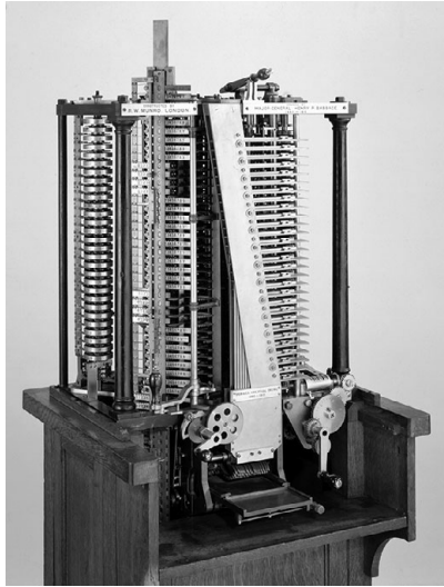
Figure 6.7 The analytical engine mill completed by R. W. Munro for Henry Babbage in 1906–10. By permission of the Science and Society Picture Library (Science Museum London 1896–0058).
