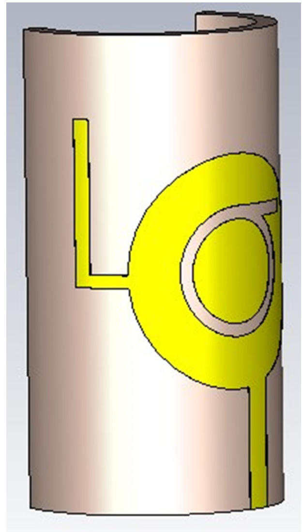
Figure 20. Antenna bent in y orientation.
