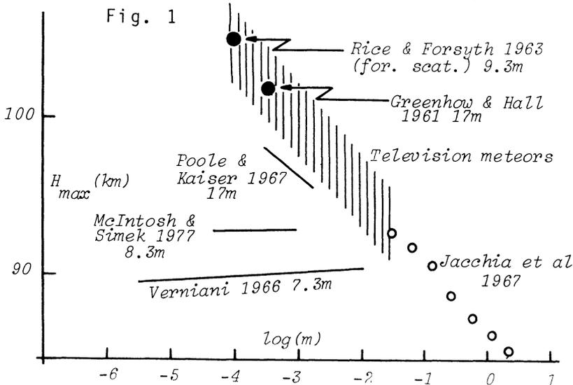
together with the data for the standard Super-Schmidt meteors and also several sets of radio meteor data. The agreement between the two sets of optical data is excellent but the discrepancy between the radio and optical data increases with decreasing radio wavelength. We will discuss this point in more detail later.
