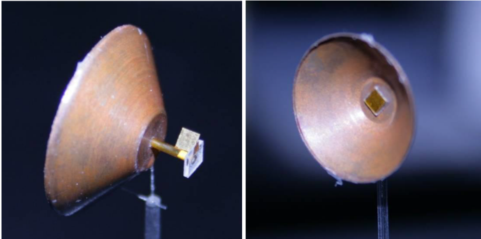
Figure 6. Images of the POLAR target from the obstacle side (left) the Au/CH pusher (right).
