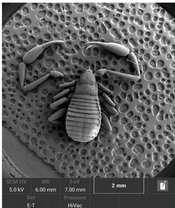
Figure 1. Large insect imaged at a single undistorted scan in FIB-SEM coincidence point (working distance 6 mm, field of view 7 mm).
