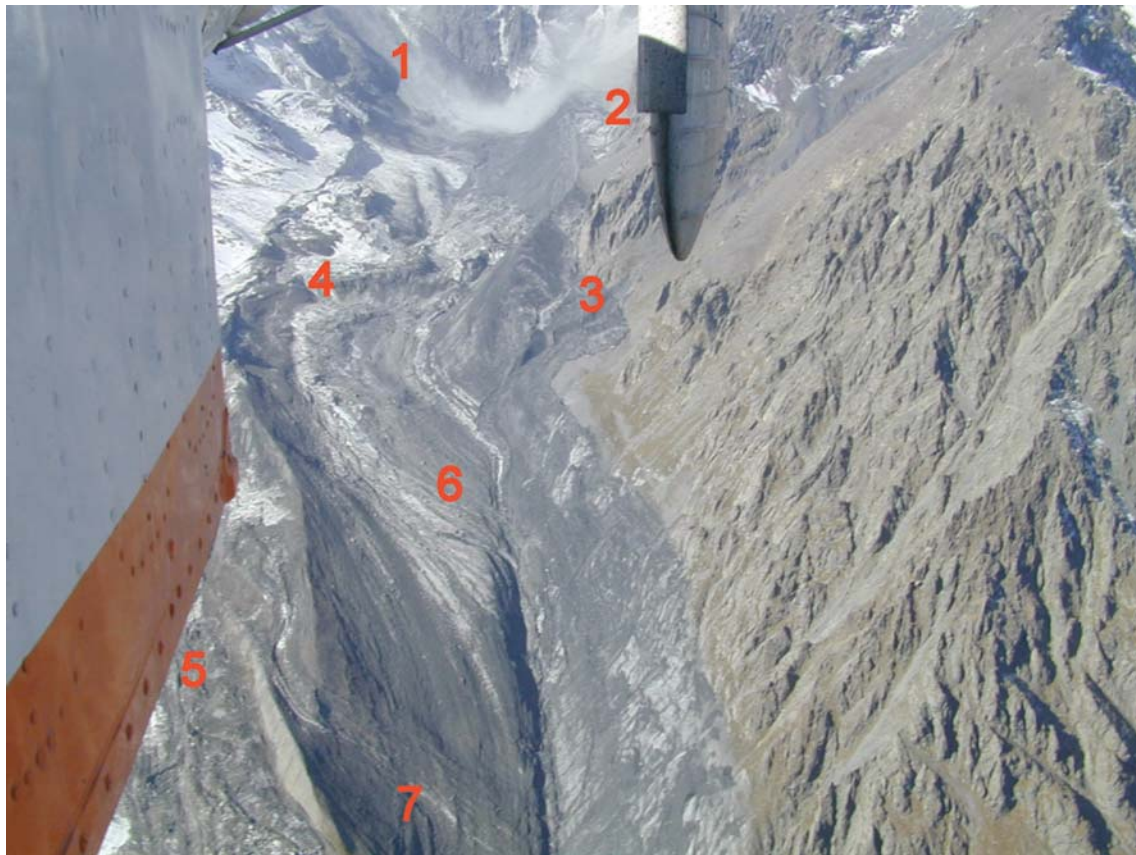
Fig. 11. Impact zone where Kolka glacier was eroded. Numbers refer to important parts of the triggering mechanism (cf. text): 1. main impact from wall; 2. ice debris thrown across left lateral moraine; 3. first (minor) splash of mud at lower end of left lateral moraine; 4. start of swing-like flow of the main mass due to deflection at left- then right-lateral moraine of Kolka glacier; 5. second (large) splash of mud forming fast mud/debris flow outside the right lateral moraine of Kolka glacier and across the tongue of Maili glacier; 6. slightly slower flow of main mass along inside of right lateral moraine; 7. temporarily blocked distal parts of fast mud/debris flow (5), crossing gap between right lateral moraine of Kolka glacier and left lateral moraine of Maili glacier and flowing across traces of main mass after its passage. Photo: I. Galushkin, 25 September 2002.
