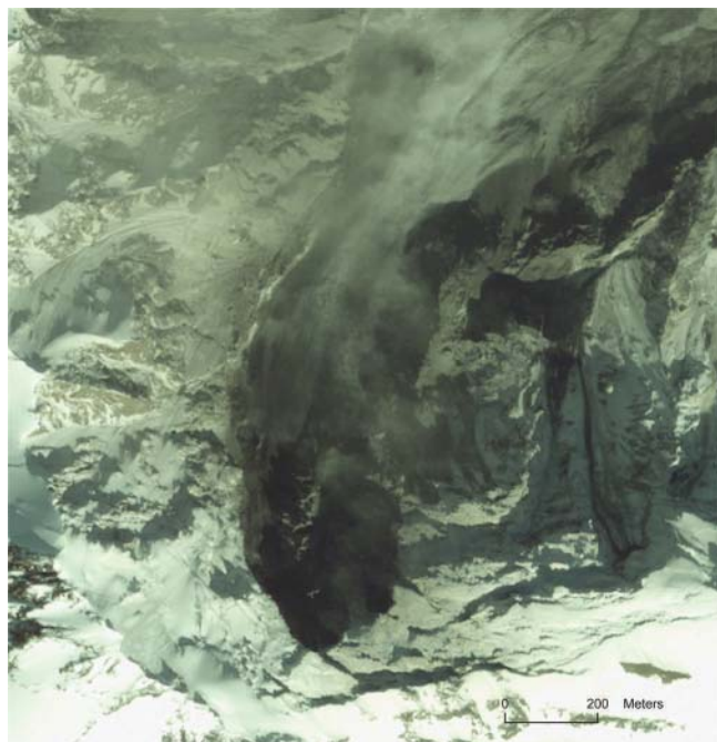
Fig. 7. Detail of the detachment zone from QuickBird image of 25 September 2002. Note black traces of rock instability to right of the dark starting zone of the main event.
