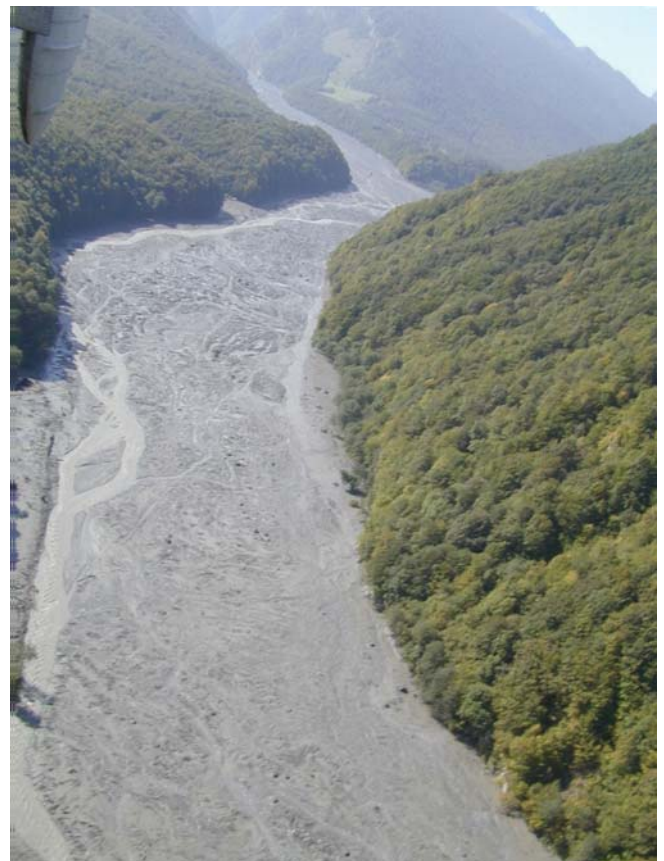
Fig. 15. Mud-flow below the Genaldon gorge. Note completely covered river bed, eliminated forest stands and buried access road. Photo: I. Galushkin, 25 September 2002.
