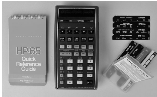
Figure 14.5 An HP-65 with its quick reference guide and magnetic program cards. Image © Whipple Museum (Wh.4529.227A).
