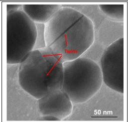
Figure 2. ADF STEM image of Au nanoparticle seeds that exhibit twin structures.
