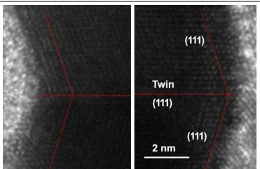
**Figure 3**. Shape of the particle and its relation to twinning as observed in an HRTEM image.
