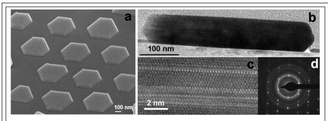
**Figure 1.** SEM (a) and Cross-sectional TEM (b) images of hexagonal Au NPs that contains twins and stacking faults. The presence of twins in the nanostructure image in (b) is also evidenced by corresponding electron diffraction pattern (d).
