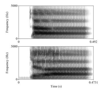
**Figure 12.** Spectrograms of sample stimuli. Top: Stimulus mirroring natural productions of high register /ta/ (Targets at vowel onset: OQ .4, BA 0 dB, FI 850 Hz, F2 1600 Hz). Bottom: Stimulus mirroring natural productions of low register /da/, with optional voicing (Targets at vowel onset: OQ .6, BA 60 dB, FI 500 Hz, F2 1900 Hz).
