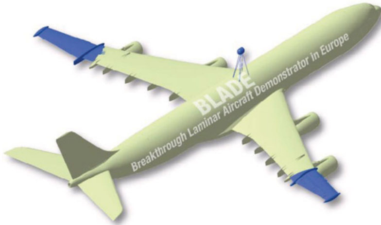
Figure 16. Modified Airbus A340 for laminar flow tests.
