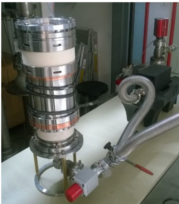
Fig. 11. Assembled inverse magnetron injection gun during bake-out process.
