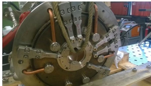
Fig. 7. Bottom view of the mirror box with the water connections for each subcomponent.
