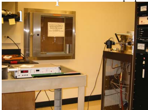
FIG. 1. The Gatan CT-3500 controller monitors the stage temperature during chamber evacuation, etching and Cr coating.
