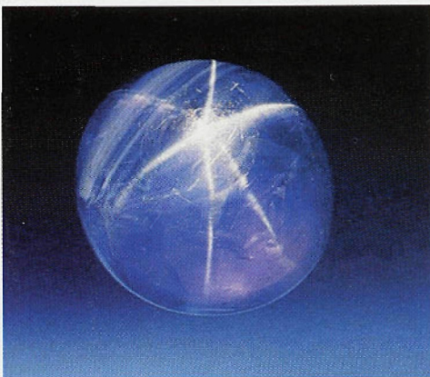
Figure 1: Illustrated are two examples of coloring mechanisms. The blue of the sapphire is caused by intervalence charge transfer while the white star is caused by scattering.
