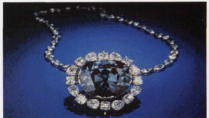
Figure 2: The Hope diamond which illustrates band gap color caused by a (natural) dopant (boron).
