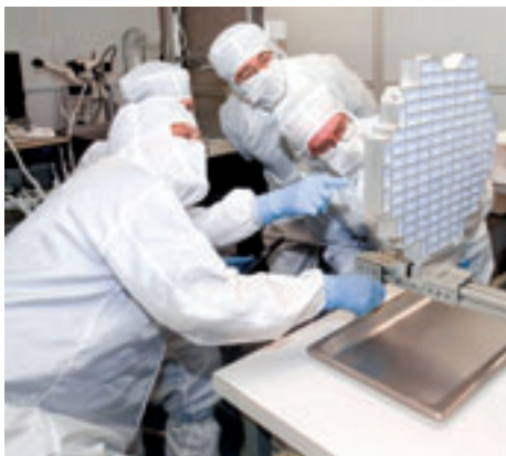
Figure 4: Scientist in the Stardust receiving laboratory at NAA/JSC huddled over the array of tiles (bluish sheen) with comet particles. Already visible to the naked eye were many tracks with the anticipated shapes of hypervelocity-impacted particles. Photo credit NASA JSC
