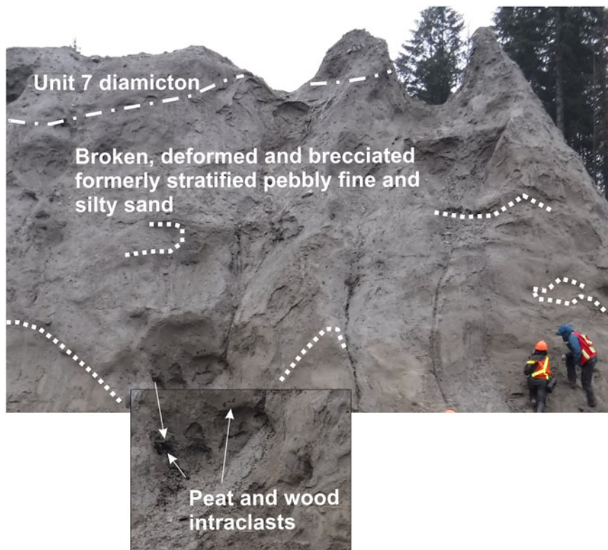
Figure 5. Exposure directly below the ground surface in the Allard gravel pit, Coquitlam (Fig. 1 (elevation ~188 m asl)), showing formerly stratified pebbly sand and silty sand deformed by overriding by glacial ice during deposition of unit 7 diamicton. It is an analog for glacioteconites intersected by drilling (e.g., Fig. 4B). The contact between unit 7 and underlying glacioteconized sediments is gradational (dotted lines define prominent deformed beds in intact blocks within the glacioteconite). Plucked peat and wood have been incorporated in this glacioteconized zone.
