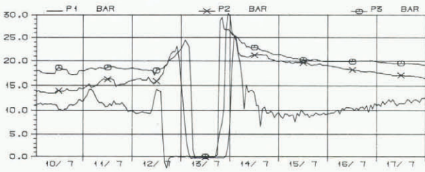
Fig. 12. Pressure recordings from a period in July 1982 when a cavity was present.
