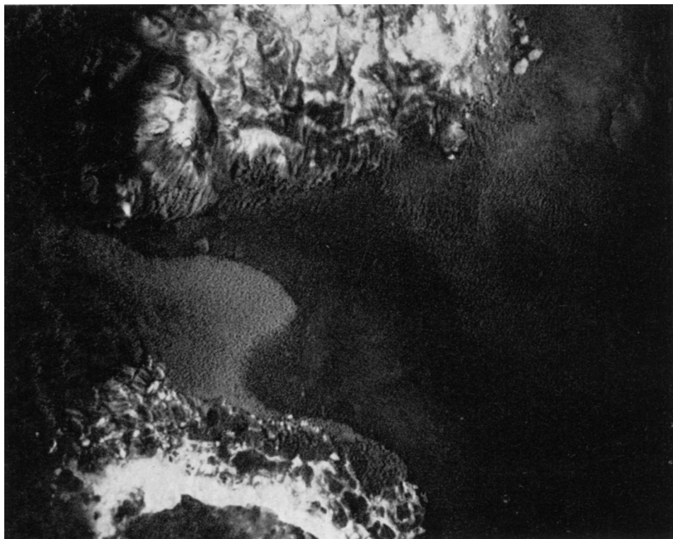
Fig. 12. Junction line formed between different materials subjected to electron bombardment in a laboratory vacuum system. The picture shows an area of approximately 4 \times 6 cm.
