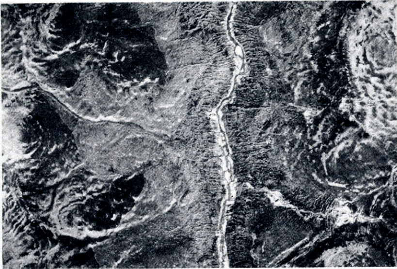
Fig. 3. Part of R.C.A.F. air photograph No. A16293-43, approximate scale 1:100,000, showing a section of the Isortoq River. The marked tonal change at the glacial lake shore-line and the light-toned areas which represent the sites of areas of former permanent ice and snow stand out clearly. The linear features normal to the river are morainic ridges with glacio-fluvial deposits nearer the river. They have a local relief of up to 20 m. Photo 4 September 1958
