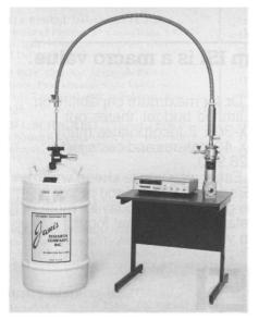
These versatile cryostats combine a flexible transfer line with a cold finger sample mount and a variety of vacuum jackets.
