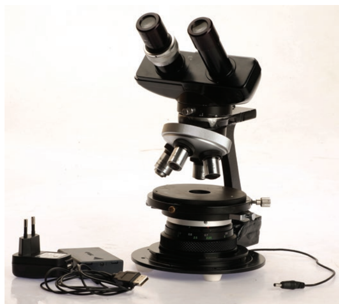
Figure 2: The portable binocular version of the microscope (photo: Pavel Shargo).
