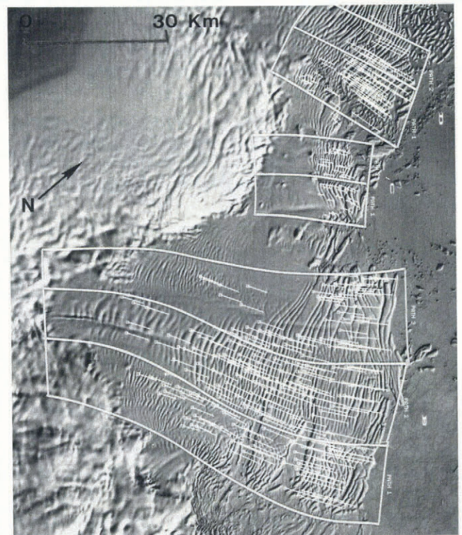
Fig. 11. Ice tongues B, C and D (bottom to top) on Riiser-Larsen Peninsula ice shelf. Displacement vectors and distances during 15.3 year period. Landsat 4 MSS image 42406-05500, 15 February 1989.
