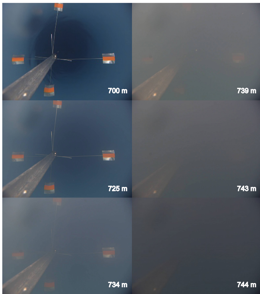
Fig. 8. Images of the water filled borehole from the downward looking camera on the clump weight on 28 December 2019 showing the transition from clear water to highly obscured over the depth interval 700–744 m. Each ‘whisker’, with an orange target is ~20 cm long. Note the significant obscuration below 739 m, which corresponds to the increase in specific conductivity in peak 1 from the 28 December 2019 profile (Fig. 6b).
