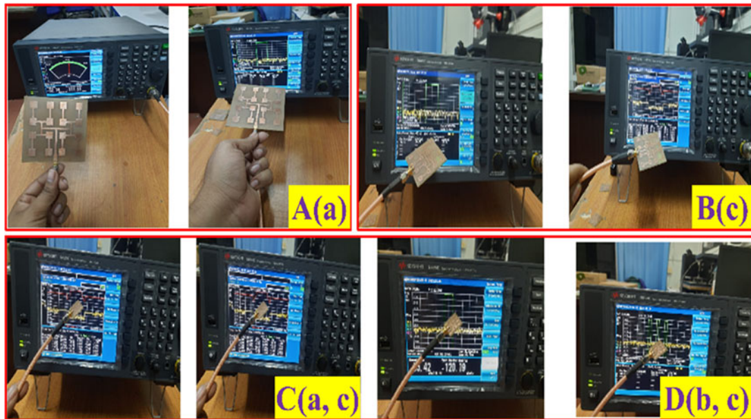
Figure 27. Measurement of different parameters and measurement setup for fabricated prototype of proposed antennae with spectrum analyzer.
