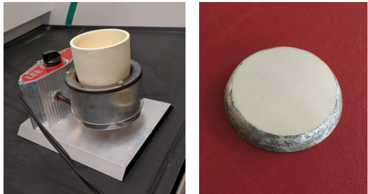
Figure 2. (a) Metal melter with alumina crucible, (b) Zn-Sn alloy sample after grinding and polishing.
