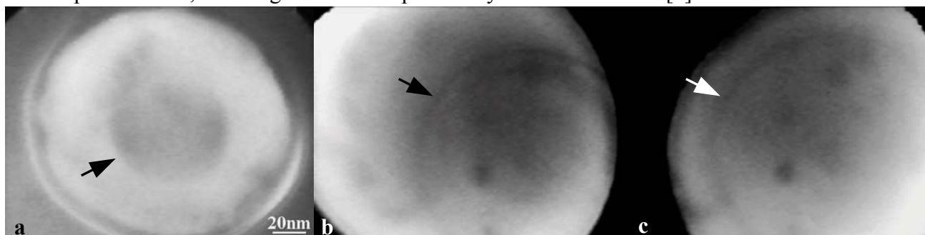
Fig. 1. Real-time in situ EFTEM video frames at 15 eV energy loss with a 6 eV window, T=658^\circ\text{C} . (a) Electron beam-assisted generation of a 40 nm diameter solid sphere (arrow) inside a partially molten Al-11.6 at. % Si particle surrounded by a \sim 10 nm thick oxide shell. (b, c) Steering of a second solid particle (arrows) by moving the beam and/or stage. Frame (b) is separated from frame (c) by 17s.
