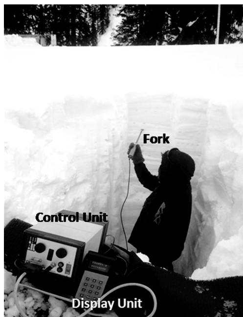
Fig. 2. Photograph of snow fork instrument during data collection.
