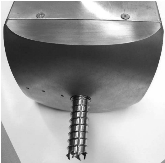
Fig. 3. IceMole 1 melting head with ice screw.
