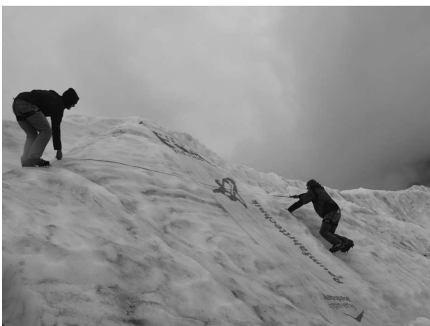
Fig. 8. Second channel melted by IceMole 1 at Morteratschgletscher in 2010: horizontal, length ~5 m.
