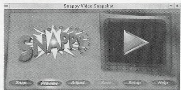
Figure 2. Snappy window in "preview" mode. Image will refresh on "TV" screen at about one frame per second for "live" focusing or other adjustments.
