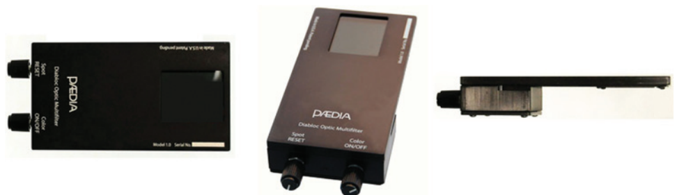
Figure 1: Top, perspective, and side views of the DOM. The Multifilter is 15 × 7.5 × 2.8 cm in length, width, and height.
