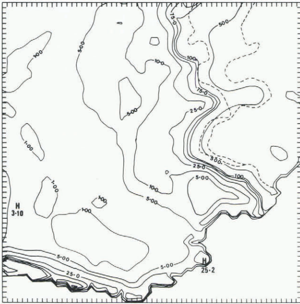
Fig.8. Sliding velocity V_s . The computed sliding velocity as derived from the sliding relation given by Figure 7 is shown with contours 1, 5, 10, 50, 100 and 500 m a^{-1} . The pattern has a similar trend of increase towards the grounding line as the balance velocities but with lower values inland.
