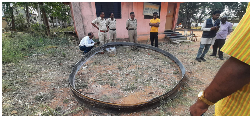
Figure 4.3 Part of a re-entered rocket body. According to Jonathan McDowell of the Harvard & Smithsonian Center for Astrophysics, who posted this photograph on Twitter on 3 April 2022, ‘This 3-meter-diameter ring is consistent with being part of the CZ-3B third stage tankage. It was found in Sindewahi (79.6E 20.3N) in eastern Maharashtra.’ See twitter.com/planet4589/status/1510658292640534534 .
