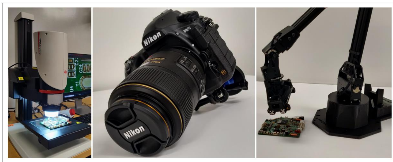
Figure 1. Figure 1: Digital Optical Microscope (left) for high resolution imagery, DSLR camera for Quick and Affordable Imaging (middle), and Robotic Arm for faster and iterative reconstruction (right).
