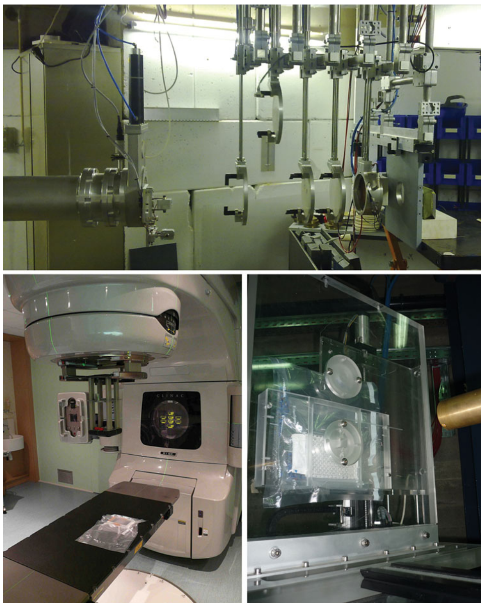
Fig. 2. Top: proton irradiation using the Light Ion Facility (LIF) at the cyclotron of Louvain-la-Neuve. The source is located on the left in this picture and the samples are placed on the right behind a metal slide with a 10 cm diameter hole. Several removable disks are placed between the source and the samples to allow the modulation of protons energy. Bottom left: picture of the facility at the Institut Bergonié where samples were irradiated with 9 MeV electrons. Bottom right: mobile device developed to ensure the ELISA plate motion during carbon ions irradiation at LNS (Laboratori Nazionali del Sud; Catania).
