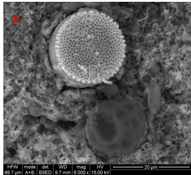
Figure 2A and B. A) Backscattered SEM images of the isolated sediment shows a matrix of circular droplets and submicron spheres. B) The recognizable shape of a diatom is seen embedded within the surrounding matrix of spherical components.
