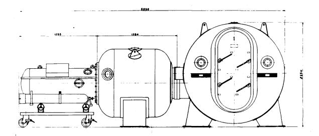
Figure 1. One-man transportable hyperbaric chamber (left) attached to stationary hyperbaric equalization capsule for personnel (center) and walk-in hyperbaric unit in hospital (right). A two-man transportable hyperbaric chamber is also available, consisting of the patient unit (left) and a transporable version of the equalization capsule for physician or technician (center). See text.
