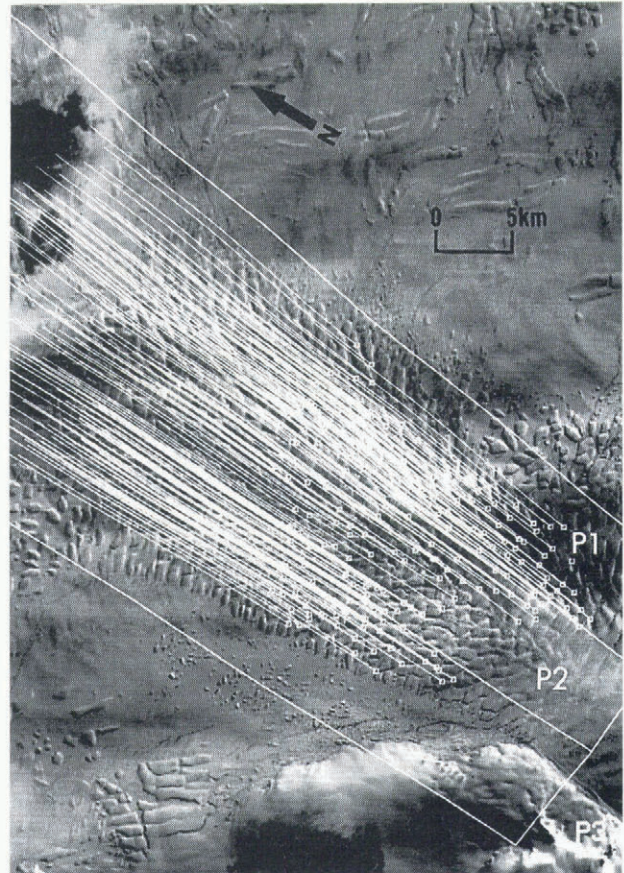
Fig. 9. Land Glacier. Heavy white lines trending north–south outline paths (P1, P2, P3); heavy white line trending east–west indicates approximate position of grounding line. Thin white lines are displacement vectors for time interval 5 December 1975–19 December 1988. Landsat MSS image 2317-16195.
